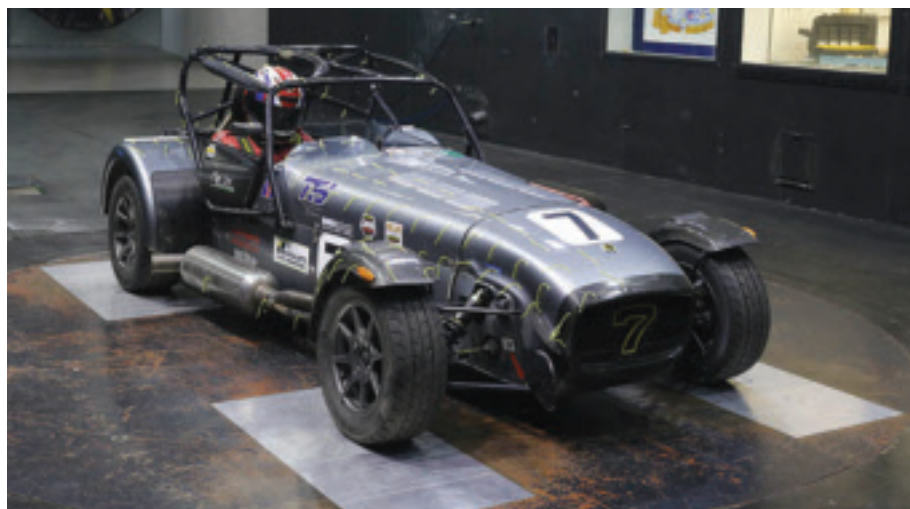
The standard S3 race car generated a large amount of lift but had a reasonable drag coefficient at 0.645. The dummy driver was used to make it as close to real life conditions as possible.
