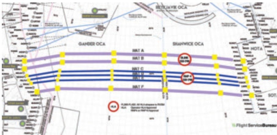
The North Atlantic Track system. The dark blue tracks are “Reduced Separation” (half tracks) for aircraft with specified navigation performance
