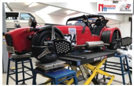
equipment. I recently took my car there for a pre-season alignment check, having had my dampers serviced, and replaced the top wishbone ball joints and track rod ends.
