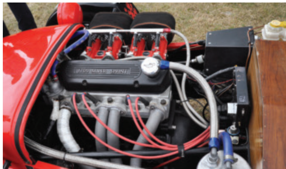
Classic Crossflow engine upgraded with OMEX ECU and fuel injection
