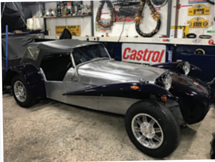
Nearing completion with its original full hood cleaned & stretched
