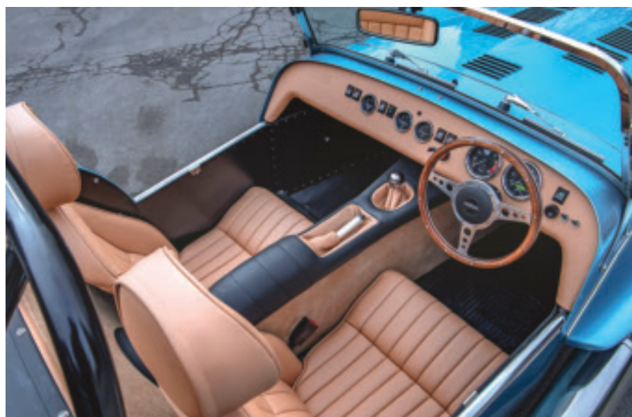
Luxury leather interior with SMITHS Instruments and wooden-rimmed Motalita steering wheel
