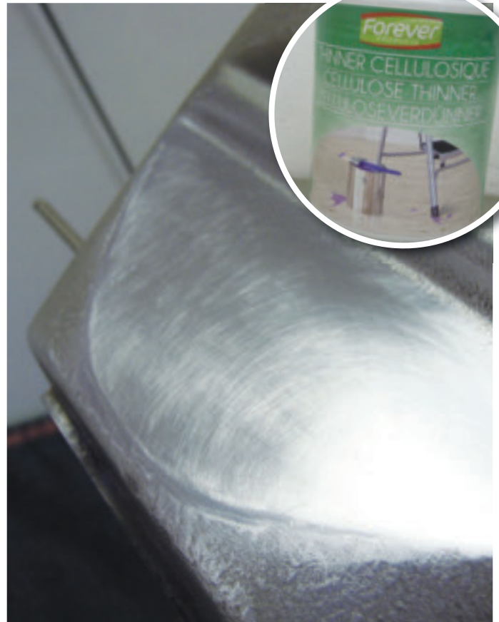
Step4: To further improve the finish, I then moved to using 1000 grid paper but with WD40 as a lubricant (main pic). Step 5: As mentioned previously, it's vitally important to degrease thoroughly (inset)
