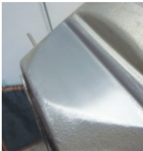
Step2: Sand with 500 grid paper. I tackled both of these steps with an oscillating sander to speed the process up. If you prefer, finer paper than 150 grit / 500 grit is OK at this stage, but may take longer! The idea is to obtain a finish that has very small or no sanding marks. When all of the coarser lines are gone, it's time to swap to a finer grade in the next step...
