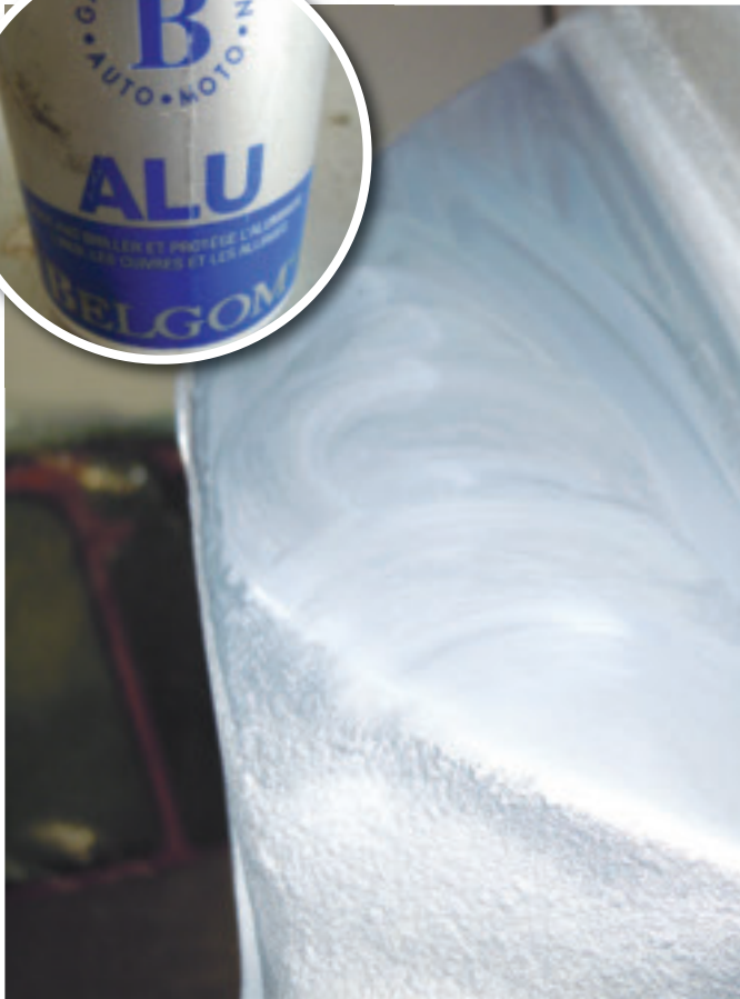
Step 6 : Polish with Belgom ALU until the alloy looks pitch black.
