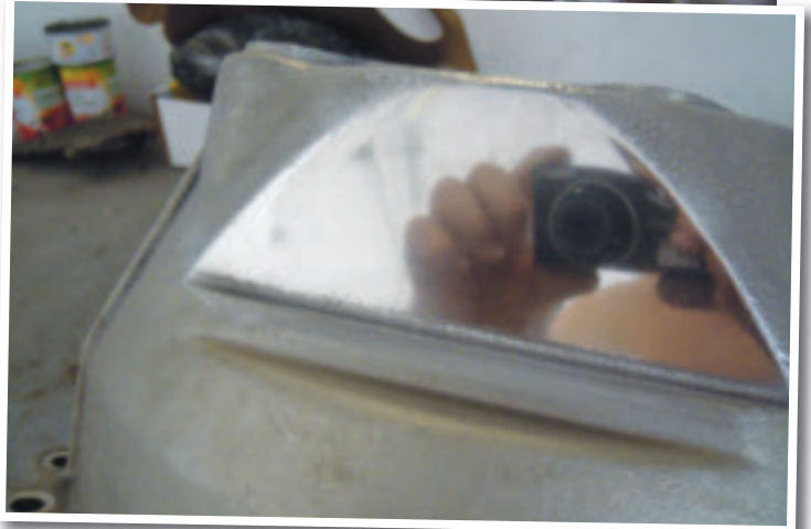
Step7: Clean the black stuff away with paper, and hopefully a mirror finish will be revealed! LF
