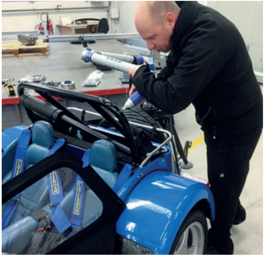
HORIBA-MIRA Project Engineer Karl Boak carrying out measurements to create an engineering model of a trackday rollover bar. For those "in the know", the rollover bar geometry was measured using a Faro Platinum 8ft FaroArm for transfer to the modelling team. The models were constructed with Altair Hypermesh and the analysis completed within LS-Dyna.
