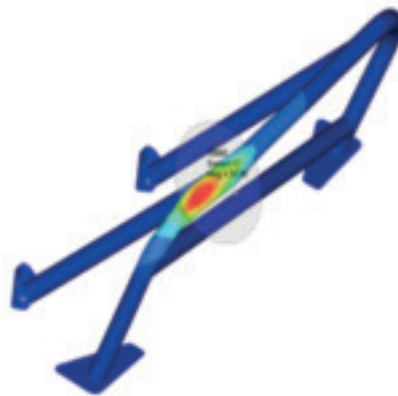
The same engineering model lifted from one of the simulated test runs, showing areas and degrees of displacement and distortion as load is applied (a 'heat map' approach with red representing the area of highest displacement)
