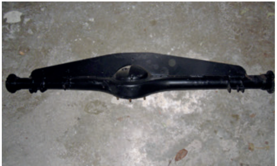
The Ital Axle as prepared for the Caterham application, showing strengthening plate and specific damper mounting points
