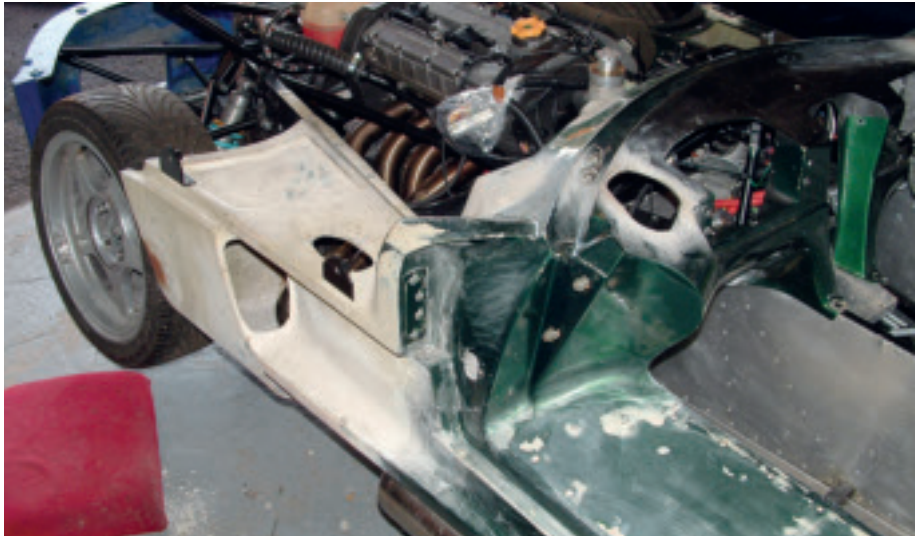
The original bodywork repairs turned out to be poor and therefore needed cutting out and restarting.
