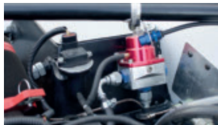
Layout of vacuum receiver, Tmap sensor and pressure regulator
