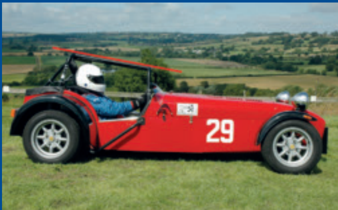
Roadsport cage, standard floor (separate side-intrusion bar also fitted)
