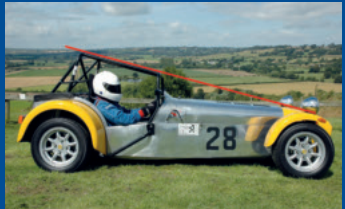
Tall Roadsport cage, standard floor (separate side-intrusion bar also fitted)
