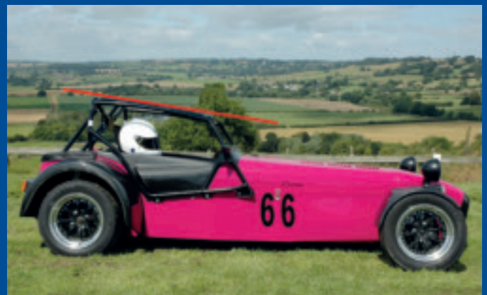
SLR cage, lowered floor
