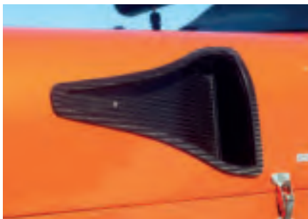
Engine breathes via a carbon fibre NACA duct, while the catalytic converter is positioned close to the engine and protrudes through the sideskin.
