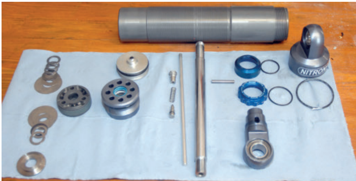
Stripped down Nitron damper. From left to right, and top to bottom: Shim stack (rebound top / compression below); piston; floating piston; gland (closes the the damper body); top jet; jet spring and needle; adjuster rod; piston shaft; adjuster assembly and pin; "top loop" spherical bearing; body cap (with main damper body above).
