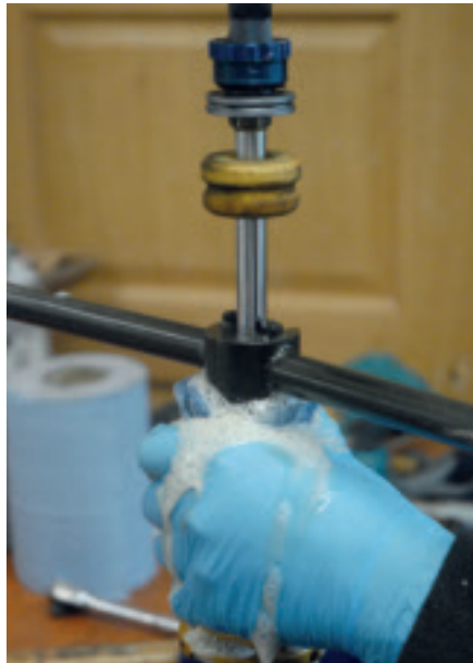
It's a gusher. The result of oil and gas mixing within a damper.
