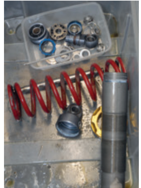
The shock disassembled and ready to be cleaned
