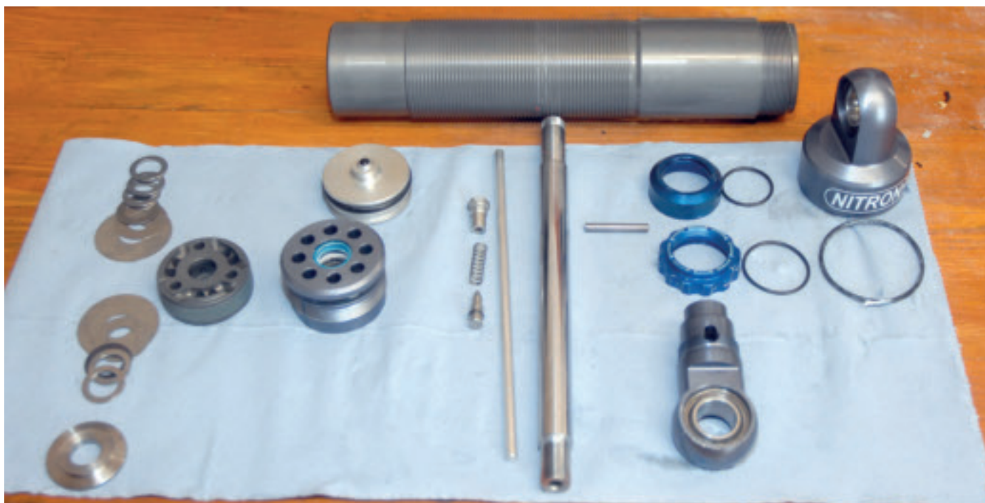
Stripped down Nitron damper. From left to right, and top to bottom: Shim stack (rebound top / compression below); piston; floating piston; gland (closes the the damper body); top jet; jet spring and needle; adjuster rod; piston shaft; adjuster assembly and pin; "top loop" spherical bearing; body cap (with main damper body above).
