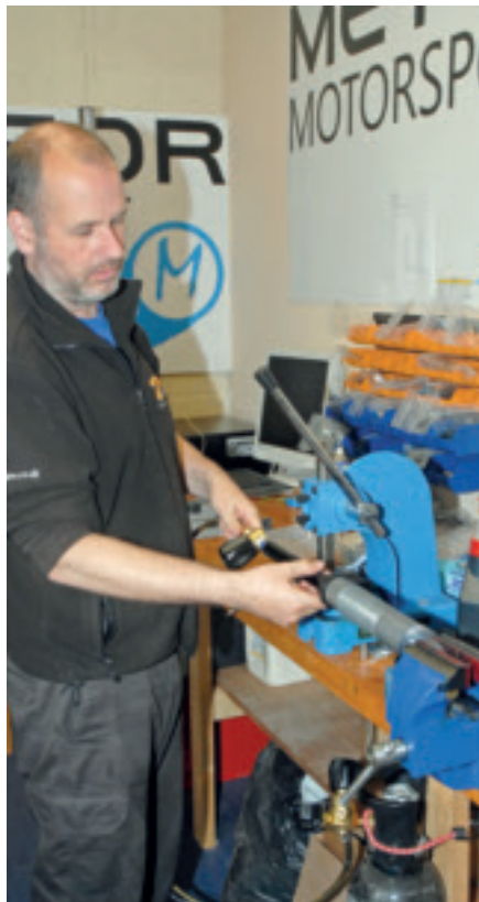
Refilling a serviced damper with nitrogen gas.
