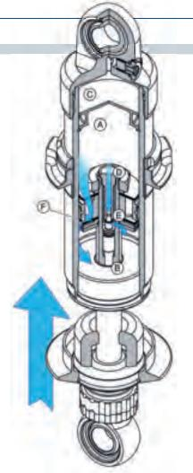
the point at which the oil is no longer able to pass through the jet alone, and instead starts to be forced through the shims. Turning the adjustment knob on most "one way adjustable" dampers has the effect of modifying the damper's behaviour in both compression and rebound, although designs where only one of these two aspects is affected are available.
