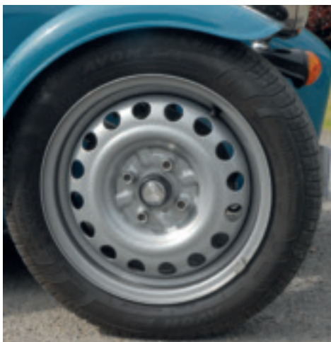
Skinny 14" Avon ZT5 fit under narrow front and rear wings
