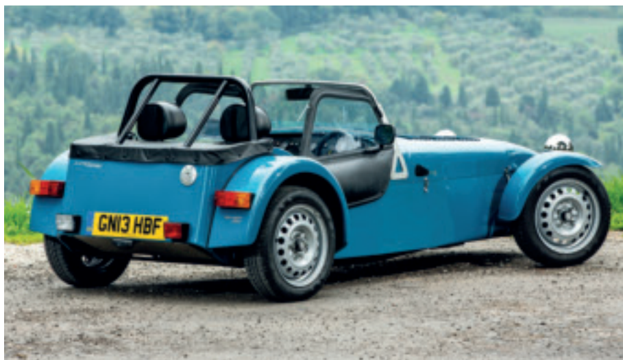
The 160 re-introduces the simple and lightweight live axle setup, not seen on new cars since the early 2000s.
