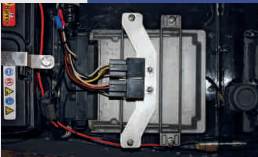
Fig 5: this is how the revised relay arrangement looks on Andrew's car.
