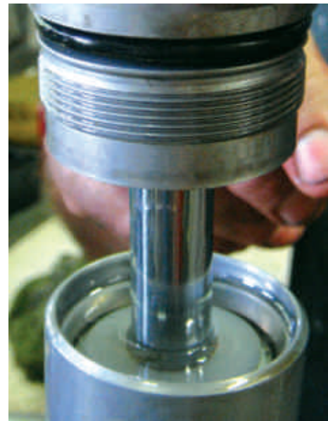
Fig 14 when raising the piston again within the body, take care not to allow air to sucked back in
