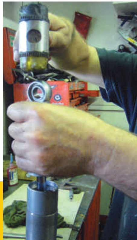
Fig 13 tapping the shaft and piston assembly with a non-marking hammer to expel any trapped air from the oil
