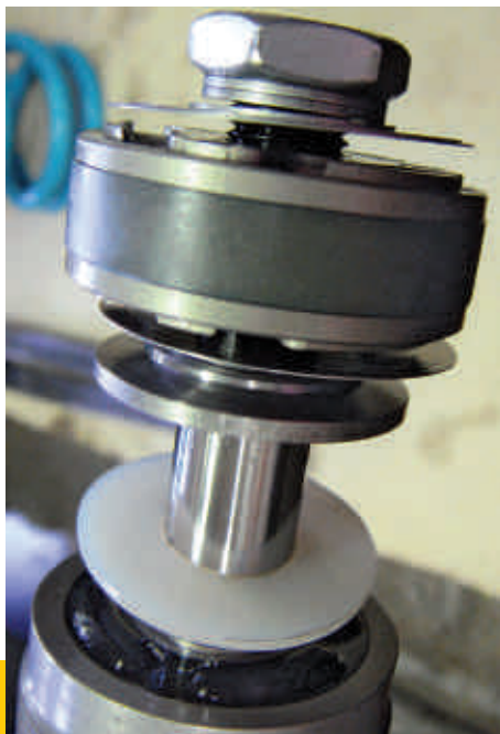
Fig 12 close-up view of the shims and spacers above and below the piston
