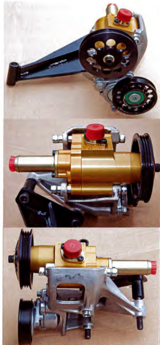
Three views of the oil scavenge pump, fitted with its pulleys and mounting bracket.
