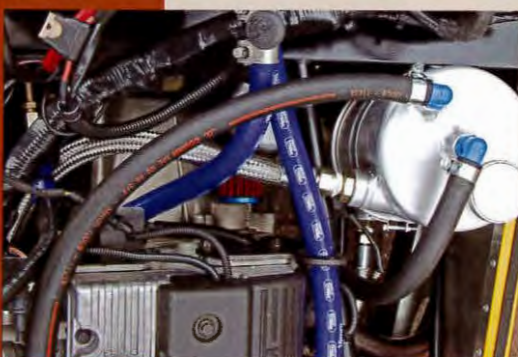
View from above, standing over front of car – showing pipe routed around bottom of engine bay and secured to chassis with rubber-lined P-clips. White circular item at bottom of picture is the coolant reservoir.
