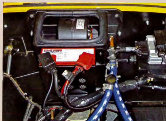
Steve's battery was previously sited in the typical spot, on top of the extended passenger footwell; with that gone, it had to be moved and his very compact Powervamp fitted on the scuttle ahead of the heater.
