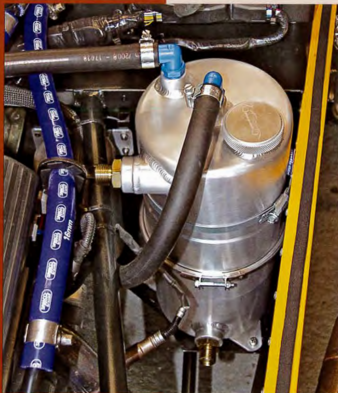
Above: The oil tank fitted into the chassis, ahead of the passenger footwell, showing the various hose connections (see text). This particular tank, the Pace Easiclean , is jointed around the middle so that it can be split in half for – as its name suggests – easy cleaning or inspection of the inside.
