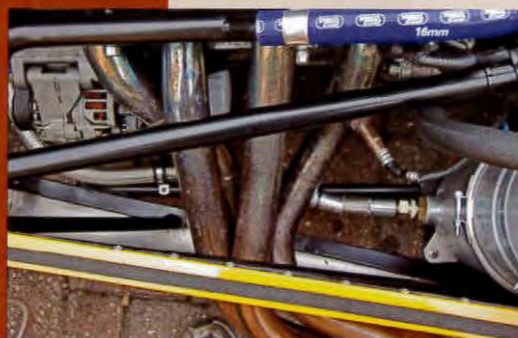
Above: The oil tank fitted into the chassis, ahead of the passenger footwell, showing the various hose connections (see text). This particular tank, the Pace Easiclean , is jointed around the middle so that it can be split in half for – as its name suggests – easy cleaning or inspection of the inside.
