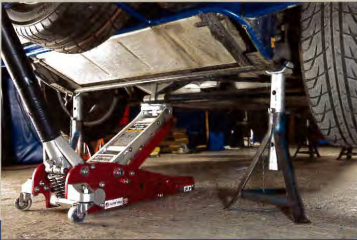
Fig 2a: S3 or SV, axle stands at rear (see detail, above right)
