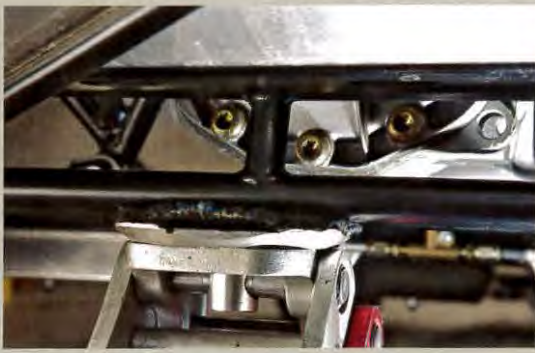
Left: saddle of jack under centre of chassis at rear of CSR.
