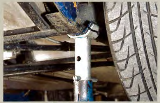
Right: axle stand supporting rear of S3 or SV (right-hand side), just ahead of the fuel tank.
