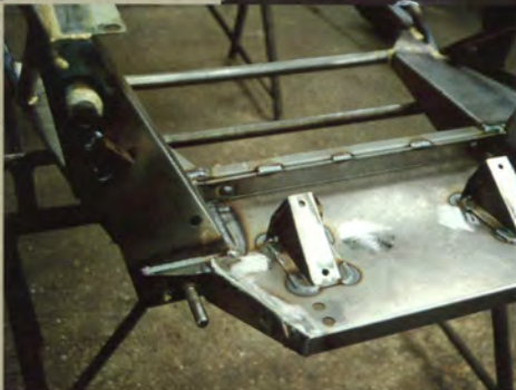
The panelled steel chassis is still available as a replacement item
