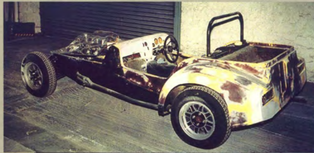
Below: refurbishment of the glassfibre bodywork is underway here, but replacement mouldings are available
