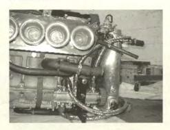
An aluminium blanking plate can be made to fit the hole left in the front cam cover by the old transverse engine mounting. Beware that you may need experiment with resizing it to get the fit correct.
