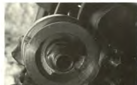
Sandwich plate fitted, showing 90° unions (viewed from beneath the car)
