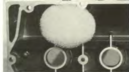
Oil union and foam insert fitted to cam cover
