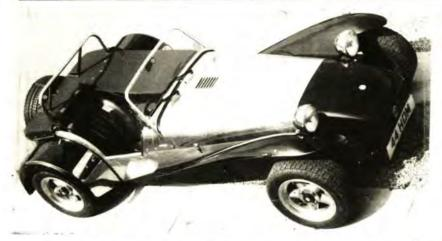
This car is a 1988 version of the Caterham. It is a standard cockpit model and uses the Ford RS2000 rear axle. The engine is a Kent 1600cc unit and has remained untouched after 86,000 miles having been 'rescued' from my previous 1980 7. The gearbox is Ford 2000E and went into the latest chassis without any alteration to the Caterham remote housing.
